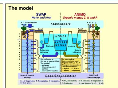
The model was set up with site specific values of hydraulic, physical and chemical properties. It was calibrated against results of groundwater level and discharge and water inlet measurements of the two-years field study.
