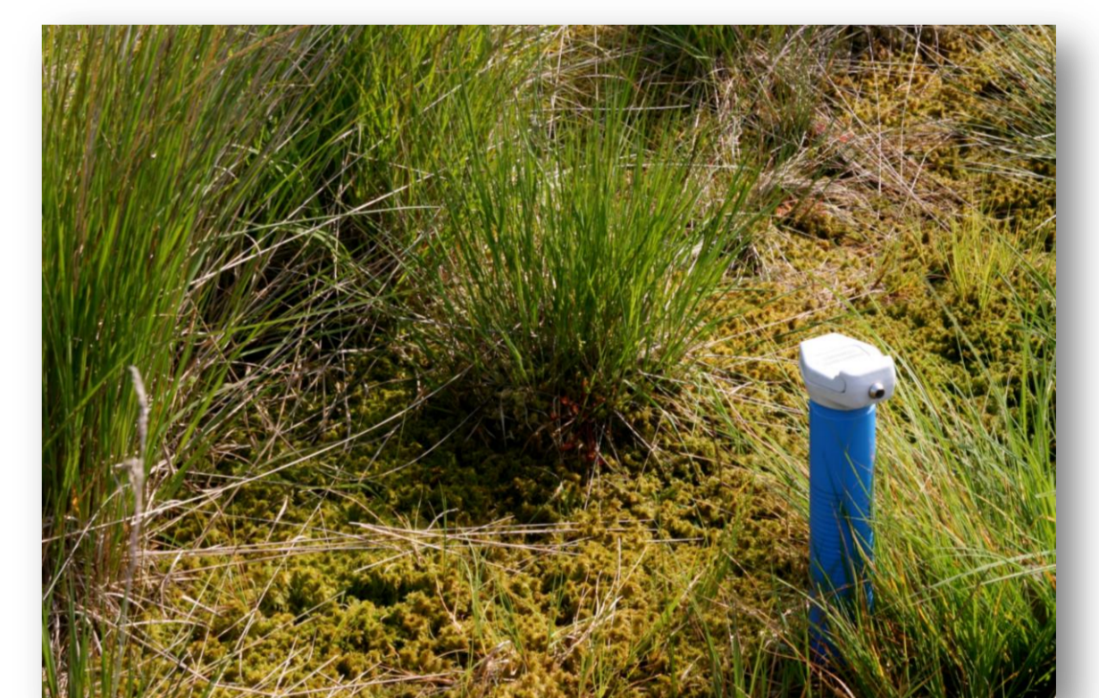
FIG 6: Groundwater level measurements in a wet grassland on bog peat.
