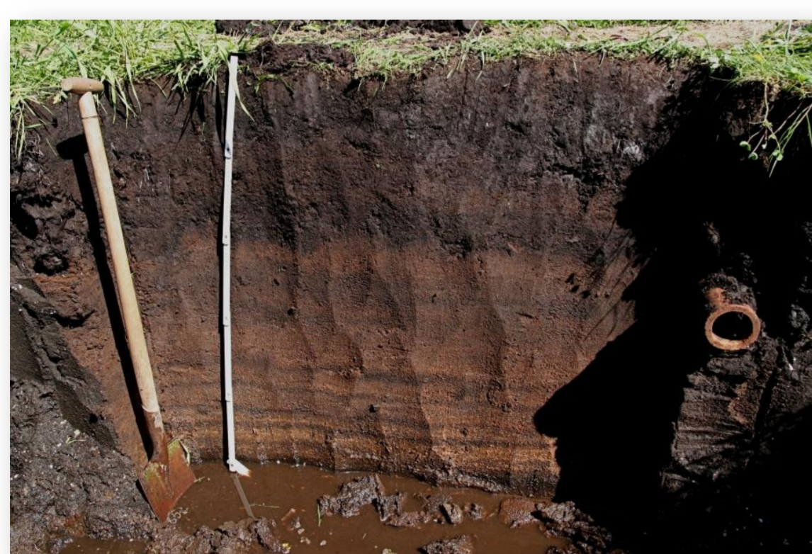
FIG 5: Profile of a peat soil degraded by tile drainage.
