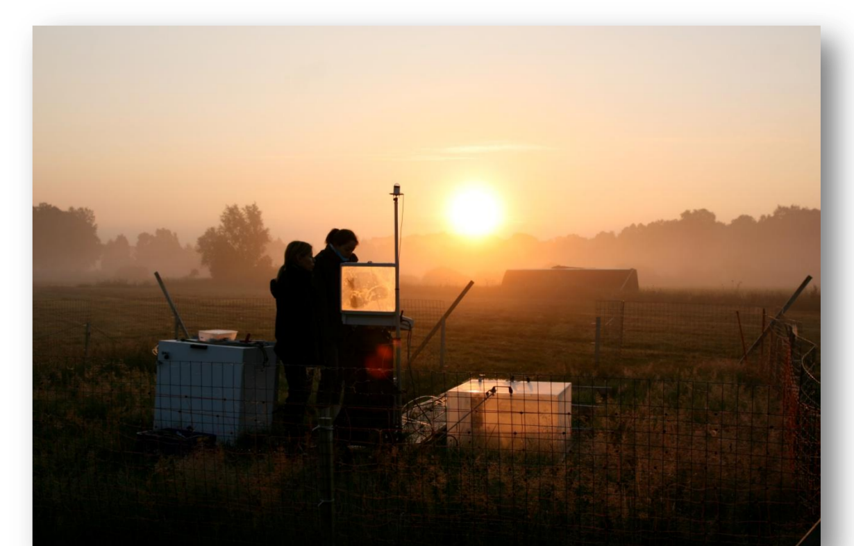
FIG 8: GHG measurements with manual closed chambers.
